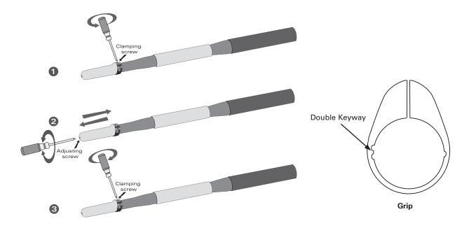
4) If the locking clamp of the adjustable grip is facing the rower's chest, remove the adjustable grip and reinstall it by aligning the double keyway with the double key. When correctly installed the locking clamp on the grip should be facing the same direction as the face of the blade.
